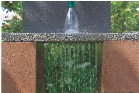
A 1 ) A Pervious Concrete Paver in Action.
